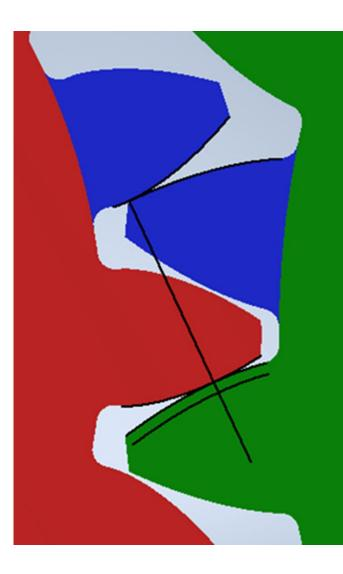
With force  $F_B$  equal to 200 and T equal to 453.1538935183, the maximum Von Mises stress equal to 20010 was determined using the finite element method.
