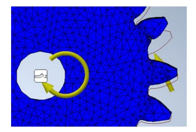
• The separation of the teeth of gear 2 is equal to the of design, the contact of the second pair of teeth will be possible and the energy will be transmitted through the two pair of teeth. Note that the contact in B will be more efficient than in E, because the radial component is smaller. Considering the mechanical errors in gear 2 with their tolerances and fits, the probability of this scenario is minimal.
